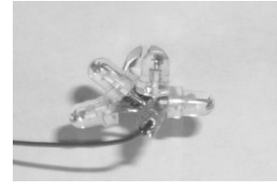
Figure 5: A set of 4 LED for direction invariant emission.
