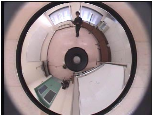
Figure 15: An example of the image obtained from the omni-directional vision sensor.
