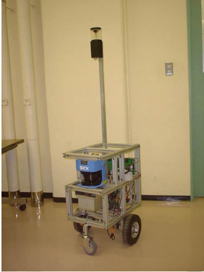
Figure 14: The robot equipped with an omni-directional vision sensor and a laser range finder.
