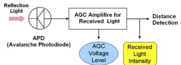
Fig. 2 Flowchart of Data Processing in URG-04LX
