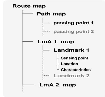
Figure 5: Route map representation separating Path map and each LmA map (Path map:Recording a passing point at the constant interval, LmA map:Recording a sensing point, landmark location and the characteristics )
