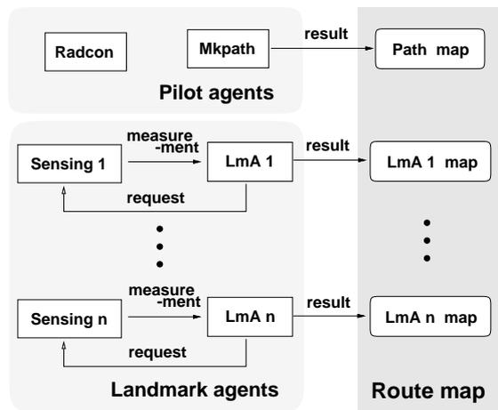
Figure 3: Multiagent programming for route map generation (*Radcon* interprets human operation at the constant interval. *mkpath* records the passing points to Path map at the constant interval. *LmA* is a landmark agent which looks for an assigned landmark and stores the detected landmark to the LmA map. *Sensing* controls a sensing direction and get the sensing results. )
