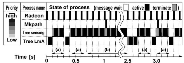
Figure 8: Time table switching multi-process as multi-agent: (a)waiting an measurement of ultrasonic range finder, (b)waiting an image processing
