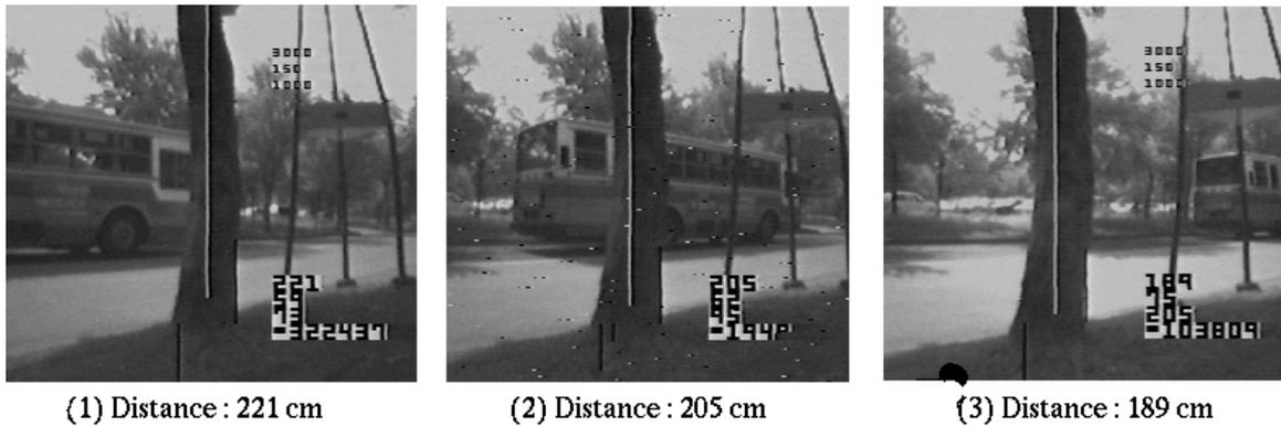
Figure 9: Tree tracking by Tree LmA (Vertical white line indicates the detected tree position in the image)
