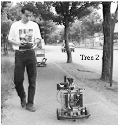
Figure 11: Photograph of route teaching (The operator has a radio controller in his hands.)
