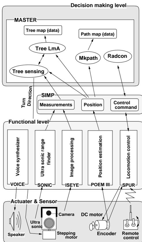
Figure 7: Schematic structure of the YAMABICO NAVI robot controllers (SIMP:State information monitoring panel)
