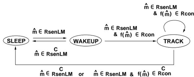
Figure 4: State transition of LmA (RsenLM is validation of the current measurement  $\hat{m}$ . Rcon is geometrical and characteristic condition to judge the same landmark.  $f(\hat{m})$  is the landmark location calculated from  $\hat{m}$ .)
