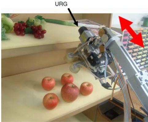
Fig. 6. Small LRF (URG) Attached to the Robot Hand.
