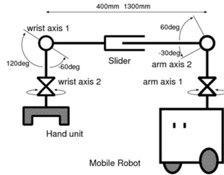
Fig. 3. Hardware Diagram of the Manipulator
