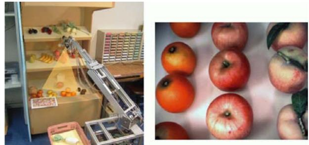
Fig. 8. Camera Attached to the Hand (left), and An Image Captured by the Hand-Camera (right)
