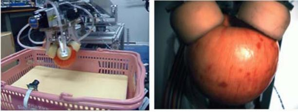
Fig. 9. Camera Attached to the Basket (left), and An Image Captured by the Basket-Camera (right)
