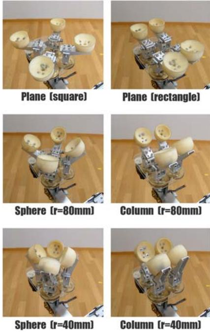
Fig. 4. Motion of the Developed Robot Hand
