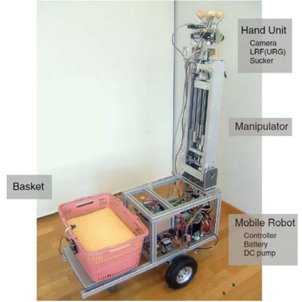
Fig. 5. The Integrated Shopping Robot
