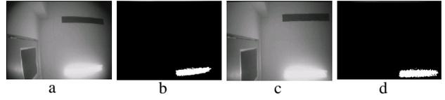
Figure 6: (a) Fluorescent light located on the border of the image. (a),(b) original and binarized images before distortion correction, (c),(d) after distortion correction.
