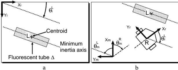
Figure 5: (a) Moment-based features of a fluorescent tube, (b) definition of the robot local reference.
