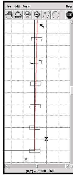
Figure 3: Screenshot of the GUI interface used to specify a path to the robot using one of the maps represented in Fig.2. This trajectory corresponds to a straight line in the middle of the corridor shown in Fig.1.a. Rectangles represent the fluorescent lights learnt during the teaching process.
