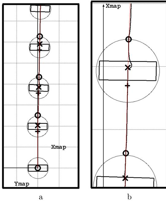
Figure 8: Odometry data of the robot correcting its trajectory using the detection of fluorescent lights in a corridor. (a) Zoom on the first lights, (b) zoom on one light. The circular disc corresponds to the light detection area. '+': light detected, 'x': *pose* correction, 'o': the robot enters a new segment.
