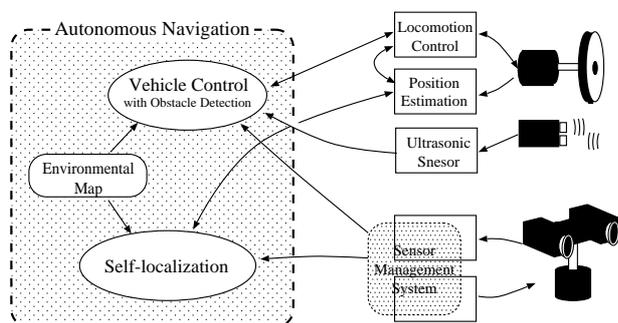
Figure 5: Structure of navigation software.
