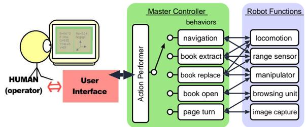
Figure 3: Structure of the software
