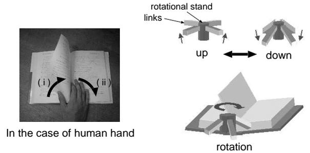
Figure 9: Structure of page turning device.
