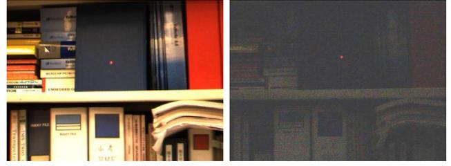
Fig. 9. The image of the laser spot light. Shutter speeds are 110ms (left) and 5ms (right).
