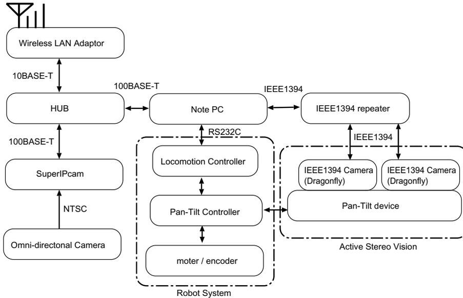
Fig. 3. Components of the system.
