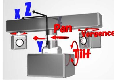
Fig. 10. Definition of a coordinate system.
