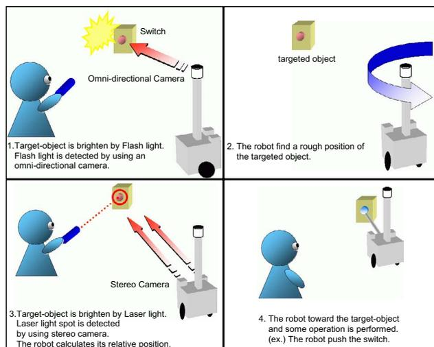
Fig. 2. Conceptualization of light projections for leading robot's navigation.
