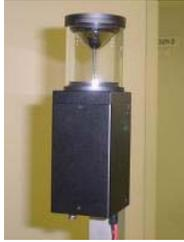
Fig. 5. Omnidirectional Camera.
